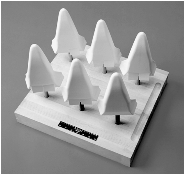
Fig. 4 The 0.0295-scale ceramic heat-transfer models.
